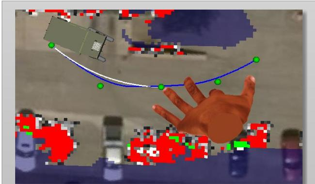
**Figure 2 – Top-down user-perspective view of realistic animated hand laying out a path for the vehicle to follow.**
